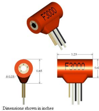
Figure 5: Frangibolt non-explosive release device.
